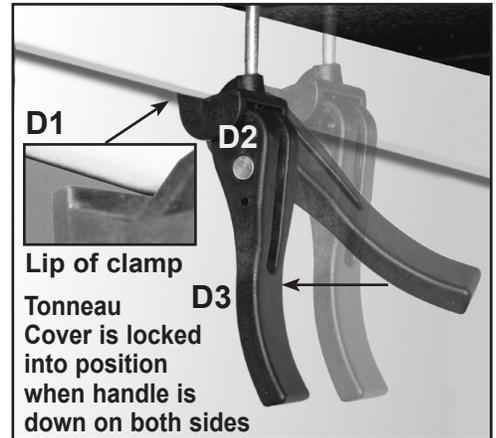
8b. To clamp cover down, put lip of clamp hooks under the side metal bed rail and push handle down. (See D1, D2, D3)
