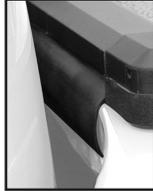
Place dust seal between cab and truck bed.
